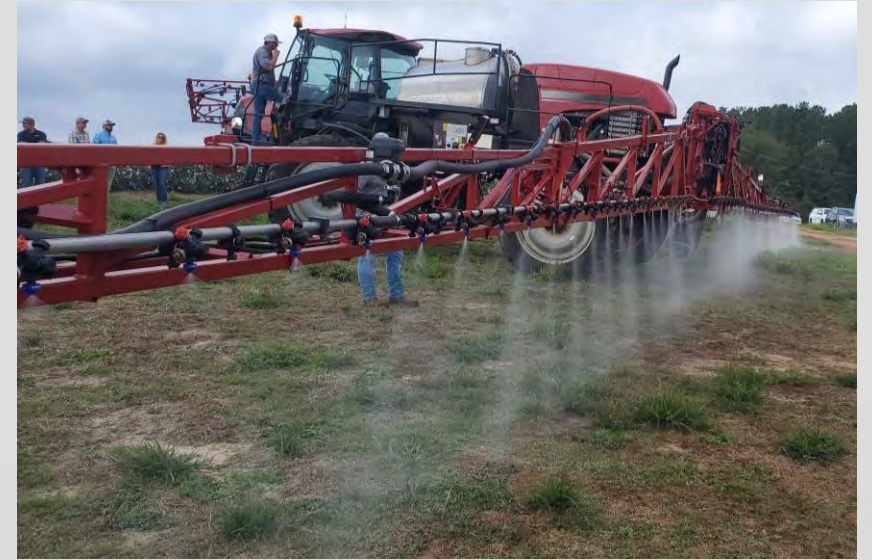
Nozzle spray pattern verification
