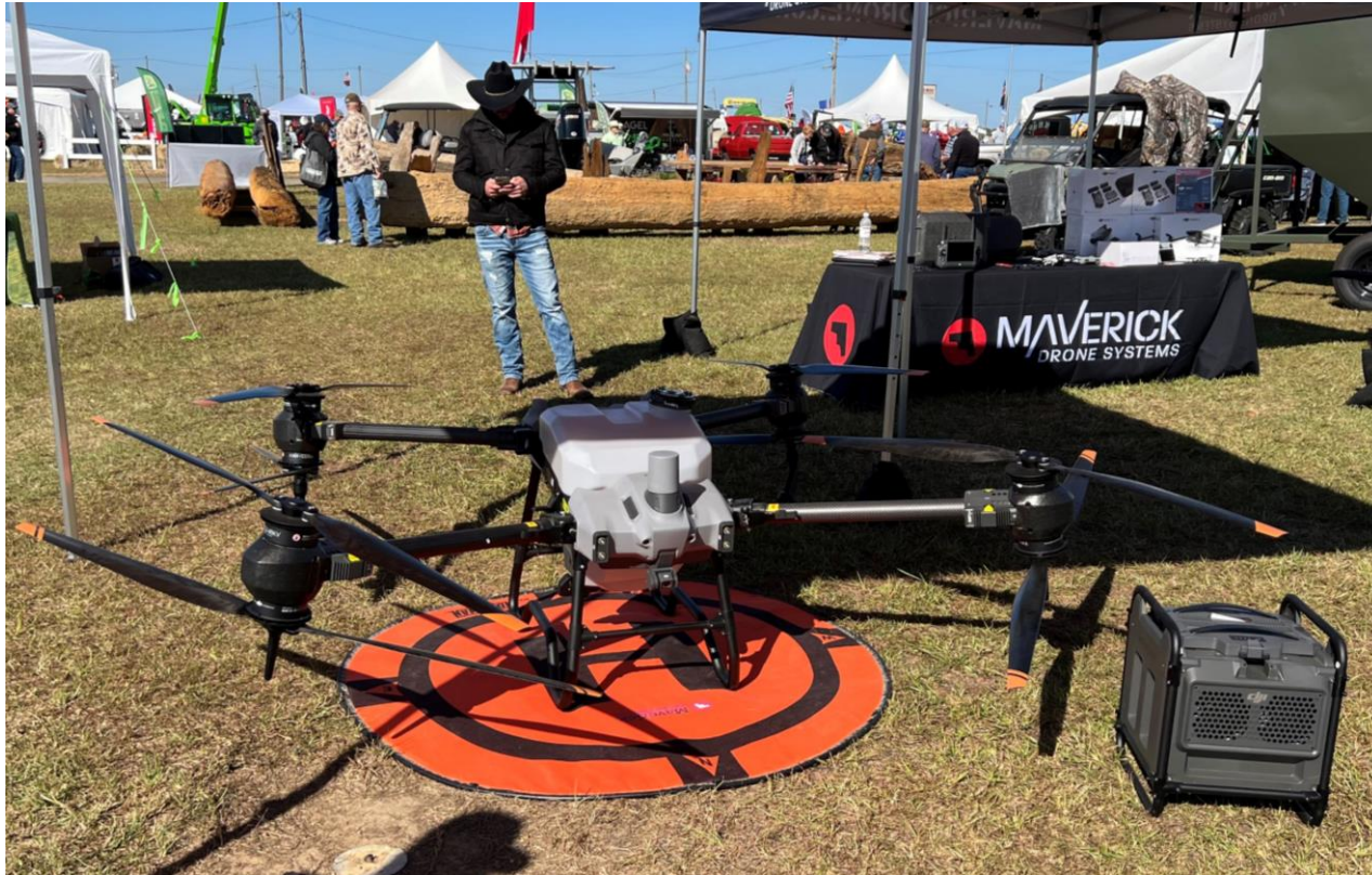
DJI T40 – 10.5 gallon tank, rotary atomizers, 36 ft swath.....
